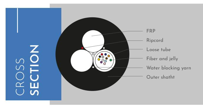
**Note:** Because the optical cable structure belongs to 3 units, the cable core structure is irregular, and the sheath thickness is relatively thin, and the surface of the optical cable sheath has certain lines.
